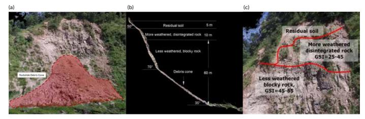
Figure 5. Characterization of a 75-m-high co-seismic rock slide in Nepal during the 2015 Gorkha earthquake. (a) 3D rock mass characterization; (b) cross-section through slide; (c) geomechanical characterization of rock mass.
