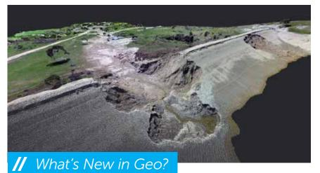
Figure 3. 3D point cloud of two failures at dam site. The left is a failure due to underseepage that resulted in a catastrophic evacuation of the impounded water. To the right, a subsequent rapid drawdown failure that occurred when the water level in the impoundment dropped.
