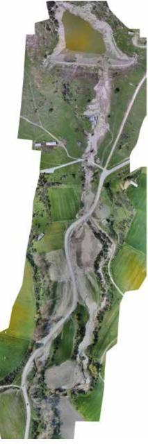
Figure 4. Orthophoto of original water impoundment area, failed dam, and flooded area downstream of the failure location. The water travelled about 1 km downstream before reaching a natural gulley and stream.
